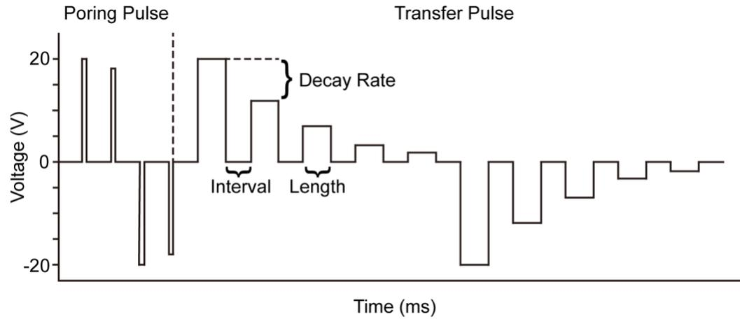
**Figure S1. Diagram of output pulses using the NEPA21 Type II Electroporator.** The diagram shows the following settings in an electroporation procedure: voltage, pulse length (duration of one transfer pulse), pulse interval (interval between two transfer pulses), number of pulses, decay rate (voltage decay rate of the transfer pulse), and polarity change.
