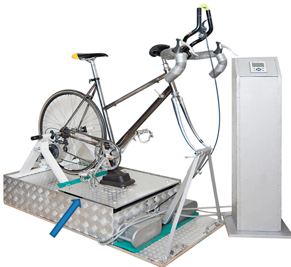
Figure 2. Photo of the vibration ergometer device used in the present study. A conventional racing bicycle was tightly mounted on a heavy platform with its bottom bracket and pedals being completely decoupled from the crank. The bottom bracket was firmly fixed to a separate plate which could be vibrated by a strong eccentric motor (blue arrow indicates where the plate with the bottom bracket is located). The bottom bracket and rear wheel were connected with a conventional bicycle chain.
